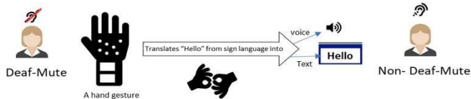
Fig: Glove translates sign language into text and voice
