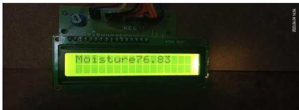
Fig 5: Output of moisture sensor
